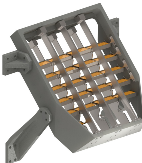
Fig. 7 Engineering design of an assembly of gratings for one (high) sector of the REDSoX polarimeter. The gratings are aligned to disperse either to the left or to the right, depending on whether the assembly is high or low along the optical axis. The gratings are stair-stepped so that the Bragg condition is met at the ML. Ribs have pins to securely position gratings below the Invar mounts and flexible arms above to maintain location.
