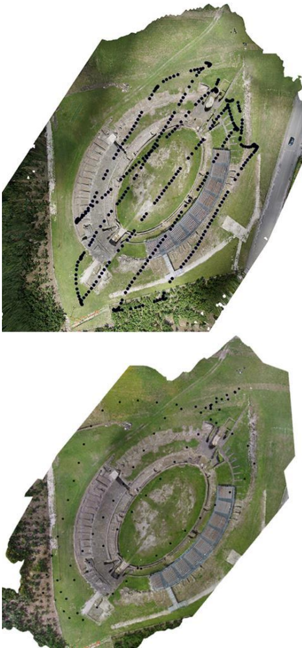
Figure 3: Nadir flight camera positions. Upper panel: hexacopter; bottom panel: DJI Phantom 3 Professional
