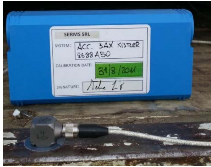
Fig.3. Picture of one of the mounted accelerometers (triaxial no. MP01).
