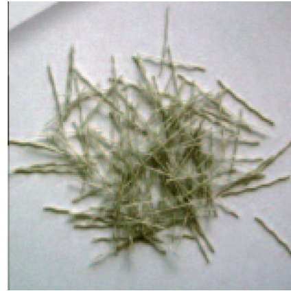
Fig. 2. The polypropylene fibers adopted for reinforcing the concrete pavement.
