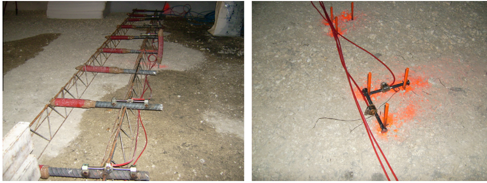
Fig. 7. (a) Arc weldable sensors (ARC) fixed to the metallic bar in correspondence of the transverse joints and (b) embedded strain gauges (CLS) to be set within the pavement. Sensor numbering runs from right to left when traveling along the lane.
