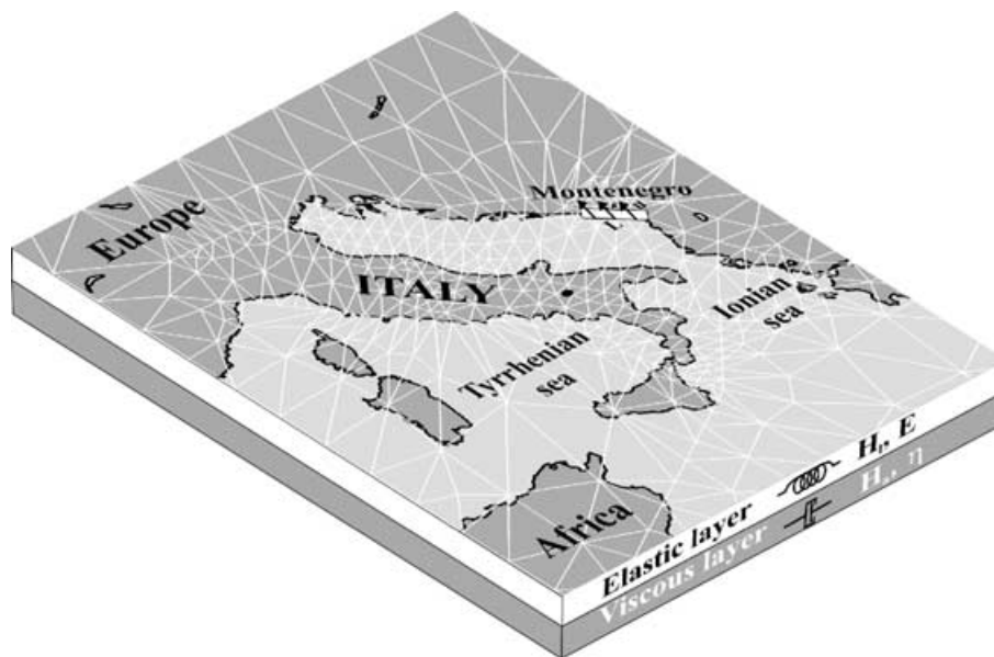
Figure 3. Model adopted and location of the fault where a displacement ( u ) is imposed to simulate the horizontal component of the coseismic slip of the Montenegro earthquake (1979 April 15 M_S = 6.7 ). The estimated seismic moment ( M_0 = 4.6 \times 10^{19} N m, Boore et al. 1981) and the distribution of aftershocks (Console & Favali 1981) are compatible with a fault length ( L ) of 50–100 km and a slip ( u ) of 1–2 m. The black dot located in the southern Apennines is the point at which the time dependence of post-seismic displacement, velocity, strain and strain rate is computed. H_l , H_a = lithospheric and asthenospheric thickness, E = lithospheric Young's modulus, \eta = asthenospheric viscosity.
