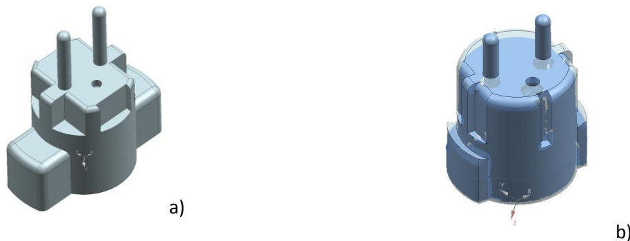
Figure 13 – Electrical Socket Adapter test case: a) Initial CAD template (grey); b) TCRT reconstruction result (grey), aligned with the acquired reference data (blue).
