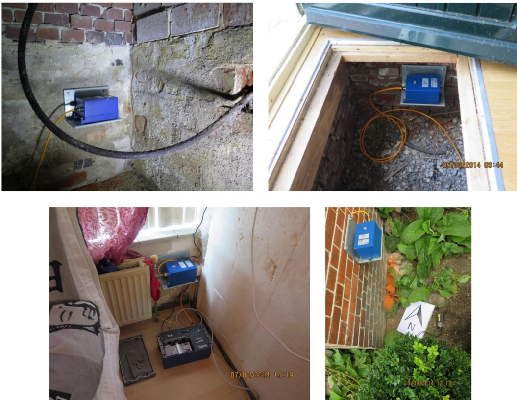
Fig. 7 Sensors installed on the walls at the: basement level (top left), crawl space (top right) and ground-floor level (bottom). Most sensors are located in the interior of the houses (bottom left), while some can be found in the exterior (bottom right)
