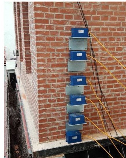
Fig. 19 Detail of the specimen house during the second shake table test at the LNEC in Lisbon (LNEC-BUILD3). Six GeoSig AC-73 accelerographs are visible: one installed on the base of the test house and five mounted on the wall at height increments of 20 cm, up to a wall height of 1.25 m
