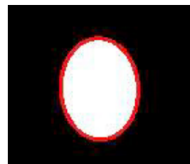
Fig. 10: Elliptical matching (in red) of the sensor boss surface (in white) with the OpenCV function fitEllipse .
