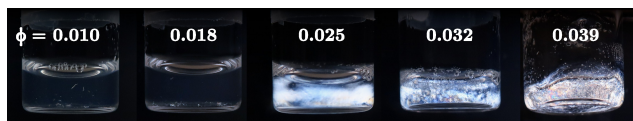
Fig. 1 Photographs of A_{10}K between cross-polarizers. For samples above roughly \phi \approx 0.02 the samples are clearly birefringent, indicating a transition from an isotropic to a nematic phase.
