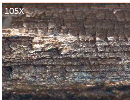
Fig. 7. Abrasion (scoring) after 2.000.000 cycles.
