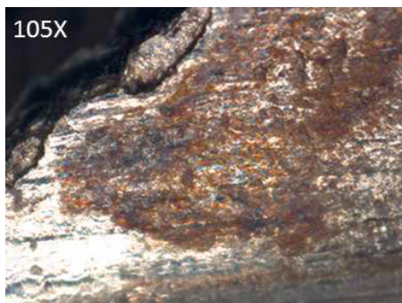
Fig. 6. Micropitting after 2.000.000 cycles.
