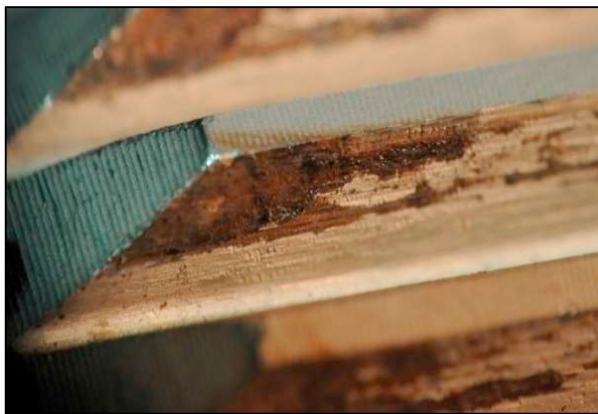
Fig. 4. Tooth area subjected to fretting wear retting wear after 2.000.000 cycles.
