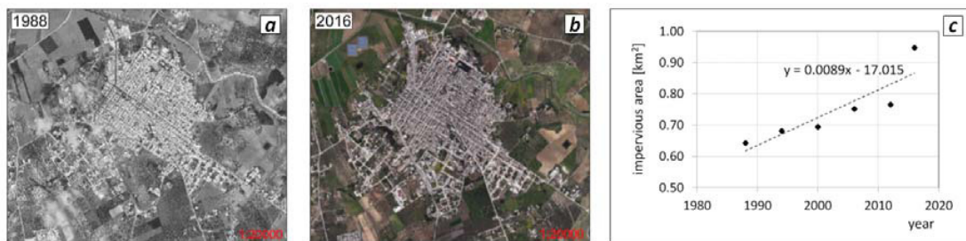
Fig. 2. (a) Orthophotograph of Paceco in 1988; (b) orthophotograph of Paceco in 2016; (c) impervious area (km 2 ) from 1988 to 2016 and related linear regression
