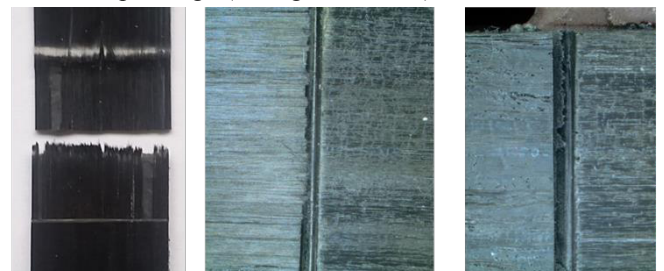
Fig. 11. Tape failure (left), incorrect slit depth (middle), correct slit (right).
