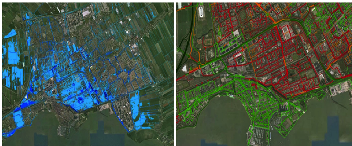
Fig. 4 Examples of different layers. Left-hand side image indicates the flooded area (blue region). The right-hand side image shows the transportation infrastructure that has been impacted by flood (red colour) (colour figure online)
