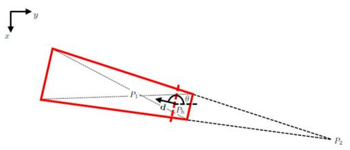
Fig. 3. Schematization of the pose estimation problem. On the Spanish fan (in red) are shown the main variables involved in the problem and the camera frame (in black).
