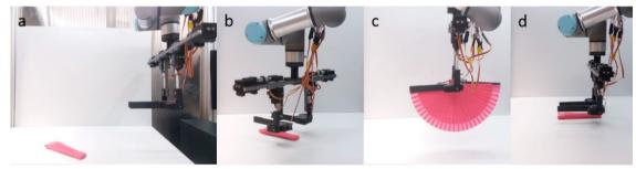
Fig. 4. Sequences of Spanish fan handling. (a) The Spanish fan is within the workspace in random pose. (b) The algorithm estimates the object pose and sends it to the UR3 arm, which moves toward those coordinates. (c) The gripper grasps the Spanish fan and handles it applying the velocities calculated in eq. 9. (d) The gripper releases the Spanish fan on the table before being moved to the starting position again.
