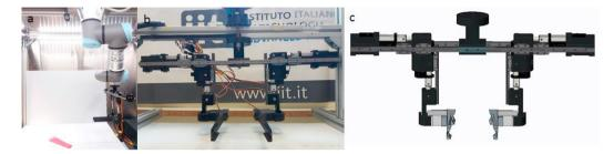
Fig. 1. (a) Experimental setup: the pink Spanish fan lays on the table, the camera and the Universal Robot UR3 are attached on top, and the gripper is the end effector. (b) Gripper prototype built with 3D printing, (c) CAD model of the gripper.
