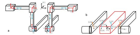
Fig. 2. (a) Gripper kinematic model: the world frame  $\{W\}$  (in black), the local frames  $\{O_i\}$  (in red), the joint velocities (in blue). (b) Dexterous manipulation problem: the twist  $\xi_i(\mathbf{x})$  of point  $P_i$  due to the twist  $\xi_E$  of the frame  $\{O_E\}$  (in blue), the twist  $\xi_i(\mathbf{q})$  of point  $P_i$  due to joint variables (in orange).
