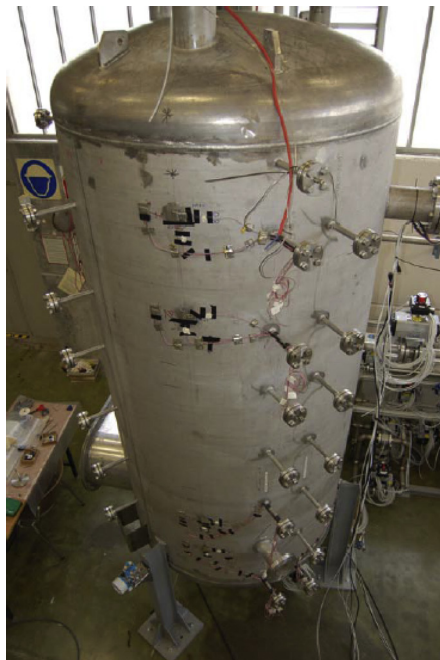
Fig. 3. CT elevation scheme with indication of the levels and types of measurement instrumentations.
