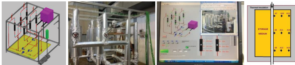
Fig. 2. ATES plant: block diagram, view, control panel for checking and ATES control and positioning of thermocouples
