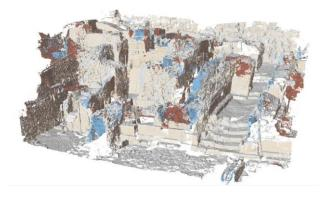
Figure 6. GoPro point cloud (RealityCapture): perspective view
