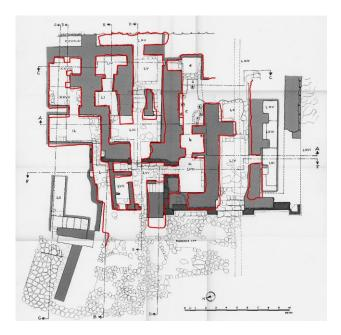
Figure 10. Overlap between the old plan and the one obtained from the photogrammetric model (red line)
