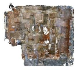
Figure 4. GoPro point cloud (Metashape): top view
