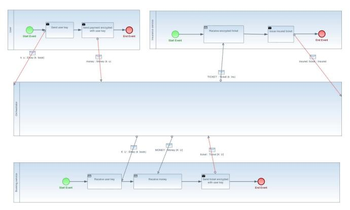
Figure 2. The BPMN specification of a collaboration diagram in which the orchestrator is represented as a black box.
