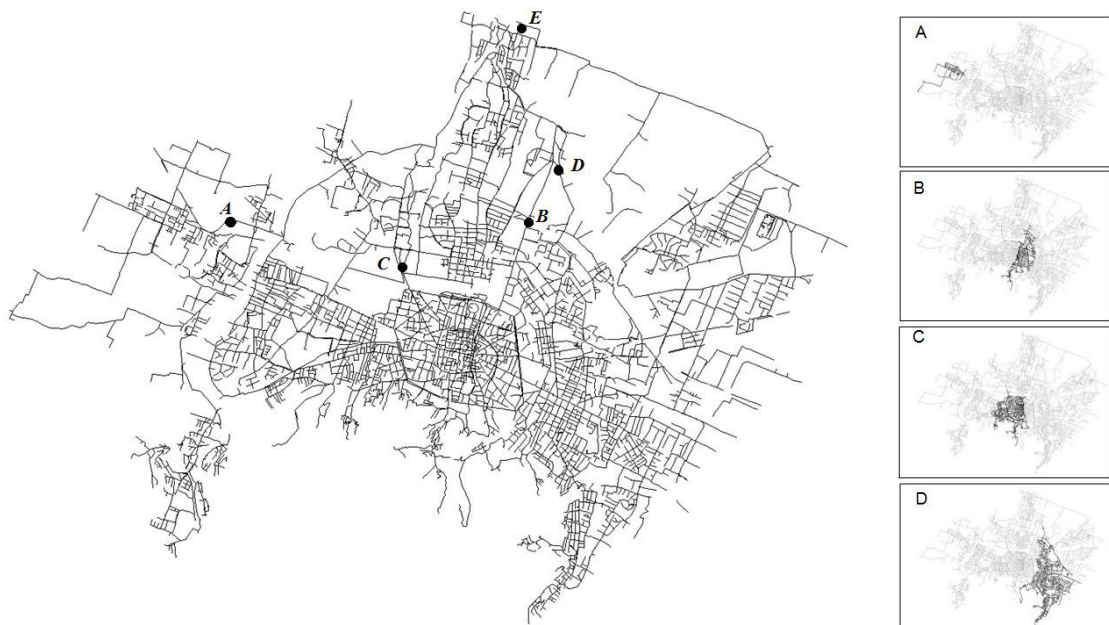
Fig. 2. Location of the measurement points with highlighted the upstream drained area for each point. The point "E" include the whole sewer system and in that point is located the wastewater treatment plan.
