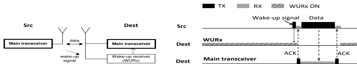
Figure 1. Implementing wake-up receivers on wireless sensor nodes
