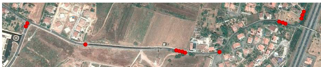
Fig. 4. Individuation of high risk zones according to DRAC values (The static information can be effective in warning drivers approaching black spots when leading vehicle is not connected).
