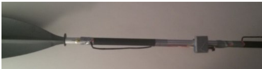
Fig. 2. Detail of the strain gage placement and the Bluetooth module on the paddle.
