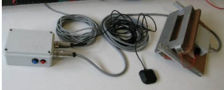
Fig. 3. E-kayak system – cabled version: control unit, foot brace and GPS antenna.
