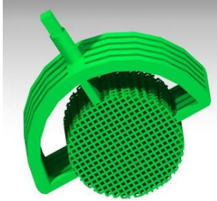
Fig. 2. Example of polymer foam used as wax pattern in the investment casting and of runners.
