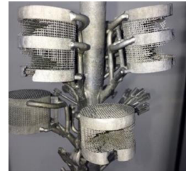
Fig. 7. Example of cylindrical metal foams obtained by investment casting.
