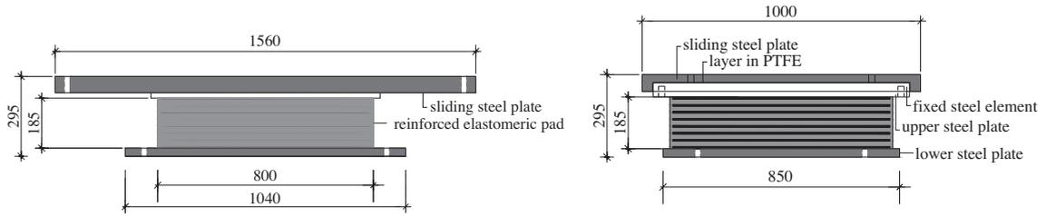
Fig. 5. Purposely designed support devices. Longitudinal (left) and transversal views. Dimensions in mm.
