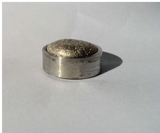
Fig. 1. Tin sample in its holder after exposure to ISTTOK plasmas.
