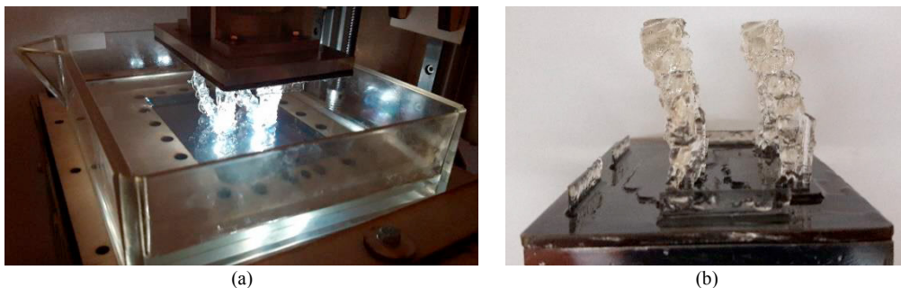
Fig. 7. (a) Phase of the 3D printing process of the orthodontic appliance showing the polymerization of a single layer by direct light projection, (b) fabricated appliances attached to the build platform.
