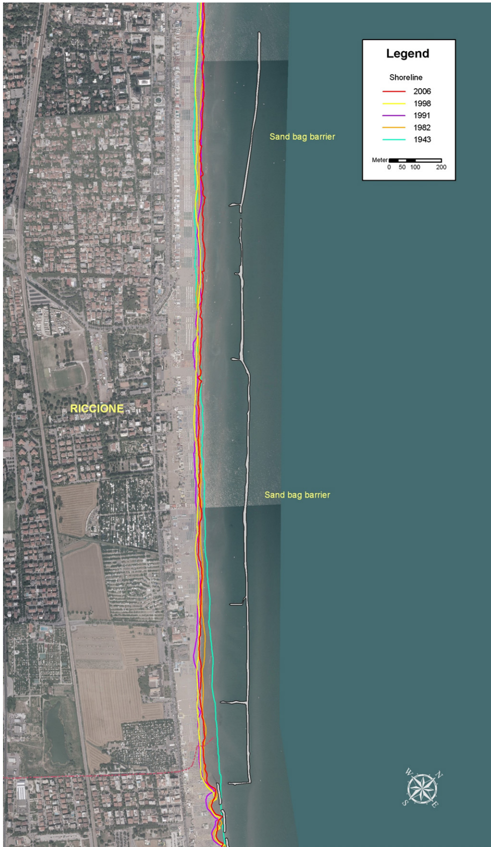
Fig. 2. Aerial view of Riccione littoral, showing the geosynthetic barrier and the shoreline evolution within the last 20 years.
