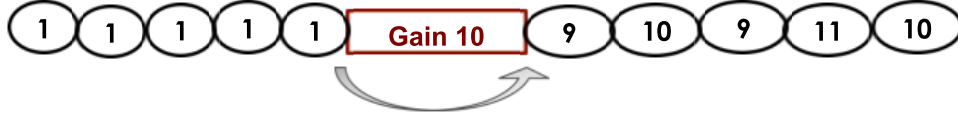
Figure 19. Excess noise factor: each unit charge entering the gain layer from the left generates a number of charges that on average equals the gain G , (10 in this case), but with a spread described by the excess noise factor F .
