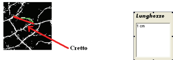
Figure 4.3: Crack length tracing
