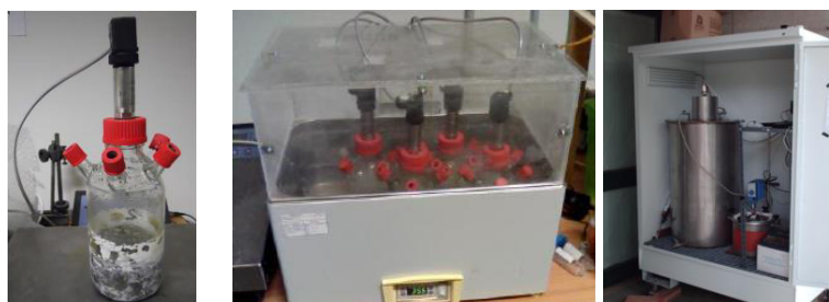
Fig.1. (a) bottle for ABP tests; (b) thermostatic bath; (c) anaerobic digester.
