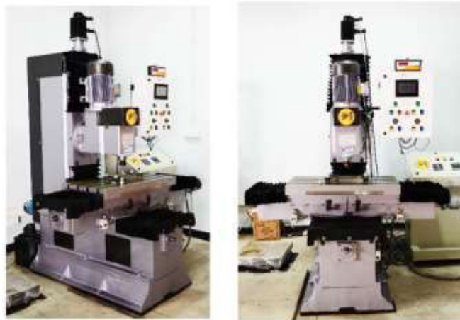
Fig. 1. Friction stir welding machine used for processing of aluminum plates.
