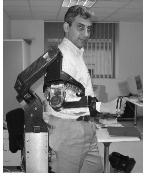
Figure 2. The PERCRO L-Exos device worn by a user.
