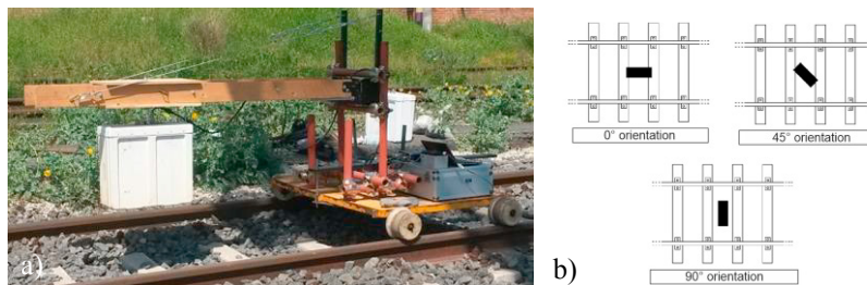
Fig. 4. (a) The experimental testing device; (b) tested antenna orientations
