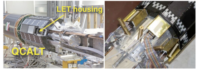
Figure 5. Left: QCALT dodecagonal structure with the LET housing in evidence. Right: QCALT structure with front-end cables in evidence.
