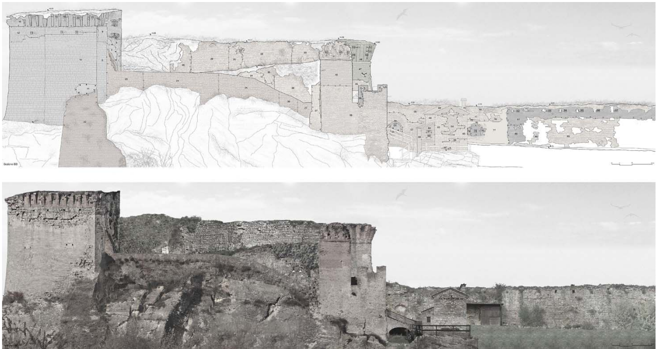
Figure 3. Castrocaro, photogrammetry and sections of S side (surveyors S. Iosca, E. Fantini)
