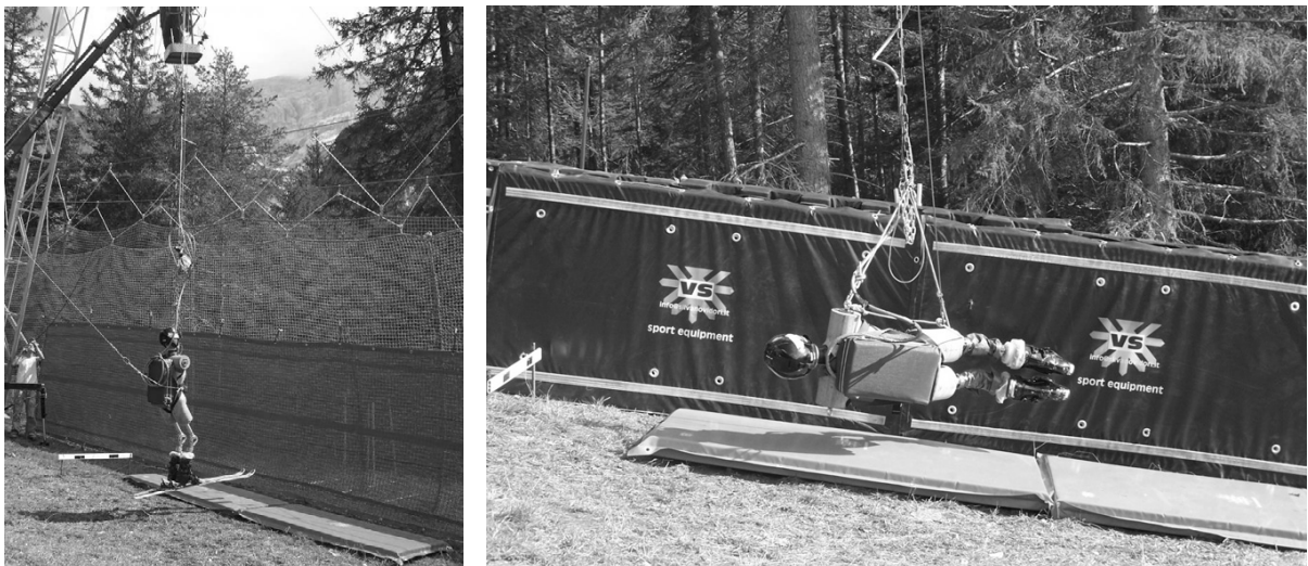
Fig.3. (a) Nets type A undergoing the test: the gliding sheet is applied to the first A1 net and the second A2 net is 1.5 m behind. (b) Foam mattresses undergoing impact tests.
