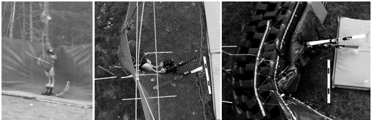
Fig.4. (a) Test Nr.22. Impact of DummyA1 wearing long skis against the SC/A1 nets: notice the extreme ski bending before binding release. (b) Test Nr.24. Impact of DummyA1 wearing short skis against the A1 net at maximum penetration depth. (c) Test Nr.29. Impact of DummyA1 wearing skis against the 1.5 foam mats at maximum penetration depth.
