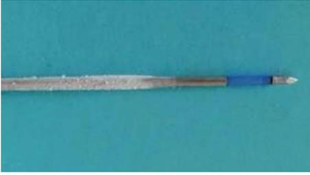
FIGURE 8: Ice crystals on the applicator's shaft surface.
