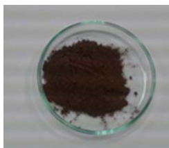
Fig. 2: The bio-residue obtained after the conversion of Arundo donax L. biomass into bioethanol.
