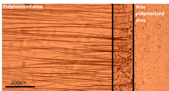
Figure 1. Optical microscope image of the fabricated pattern after the photopolymerization of MMA-PI-FeC film under external B . The edge of the laser irradiated part is evidenced between the vertical black lines.
