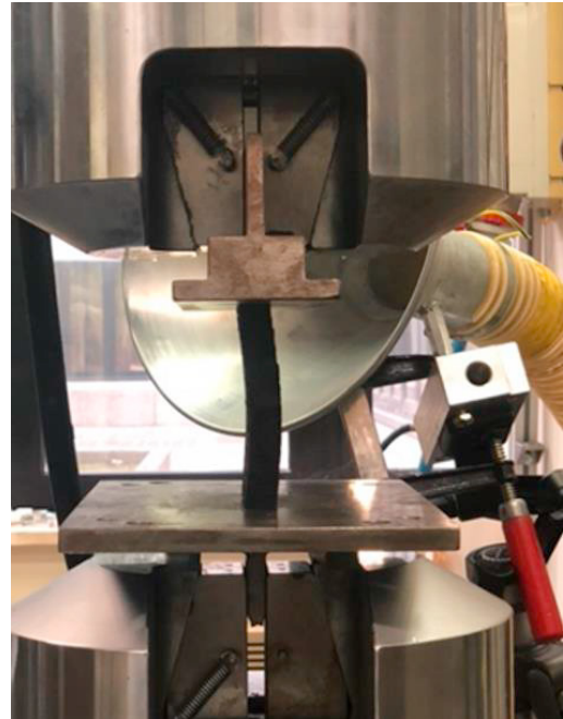
Fig. 3. Compression test of an isogrid structure in short fiber reinforced polyamide.
