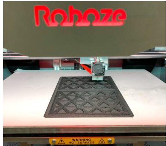
Fig. 1. The Roboze One+400 3D printer used for isogrid production.
