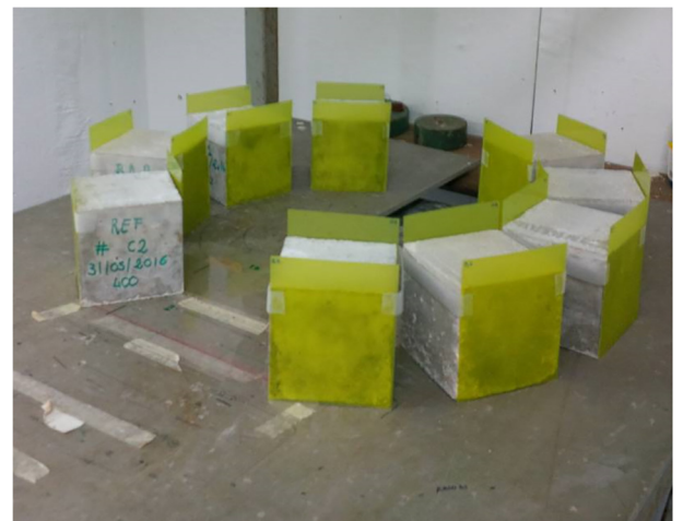
Fig. 4. Radiochromic films applied on the front and back faces of the concrete samples under investigation placed in scenario #1.
