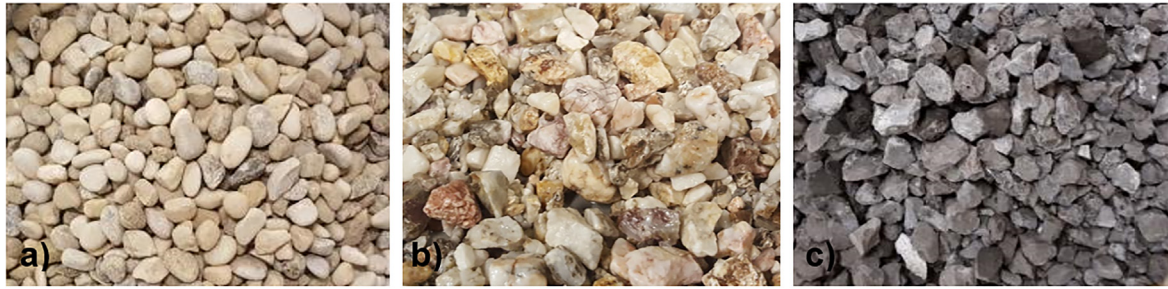
Fig. 1. a) Coarse siliceous natural aggregates; b) barite; c) EAF slag.
