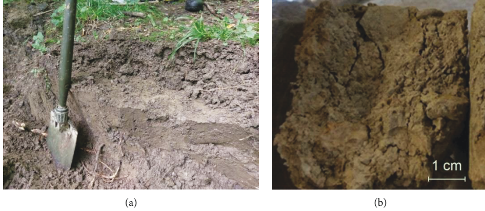
FIGURE 2: (a) Sampling pit. (b) Half of the oven-dried specimen from a depth of 0.75 m.
