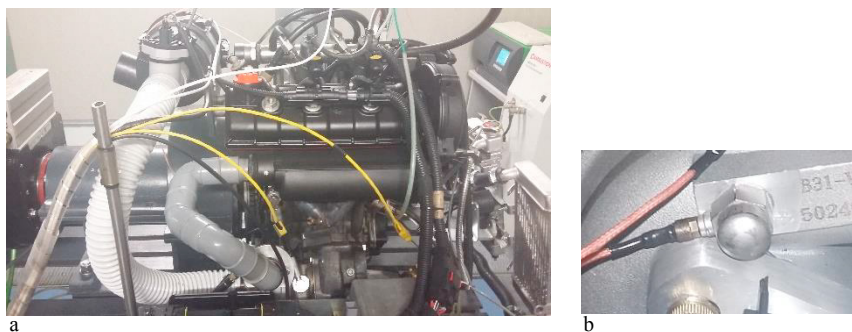
Fig. 1. (a) engine test bench; (b) accelerometer on the compressor housing.
