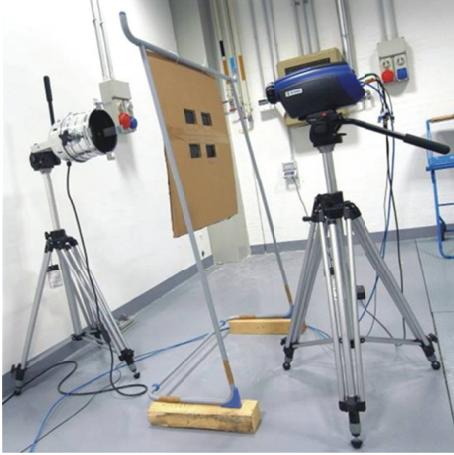
FIGURE 3: Experimental setup for the lock-in thermography in transmission mode. For the pulsed thermography, the halogen lamp is replaced with the flash lamp.
