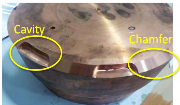
FIGURE 20. Identification with inclined reflectors: Cavity means no ultrasonic echo while chamfers means ultrasonic echo.
