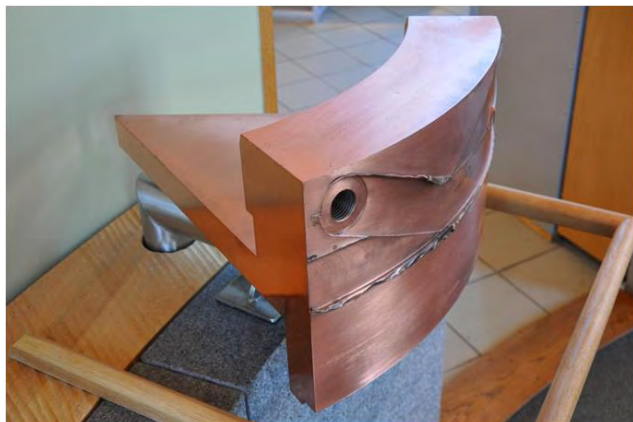
FIGURE 2. Demonstration of a piece of canister friction stir welded.
