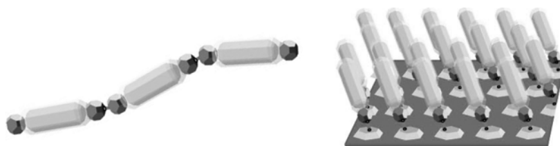
Fig. 3 Selective functionalization may be used for the formation of complex architecture as shown in a sketch here. By functionalizing only the tips of the dumbbell structures it may be possible to form chains of these particles (left sketch). This has been demonstrated already [61] by carefully exposing gold tipped nanorods to hexane(1,6)dithiol Providing functional pads (right sketch) on a substrate may enable the formation of brushes of rods. For this approach matchstick-shaped particles with only one functional domain could be of advantage.
