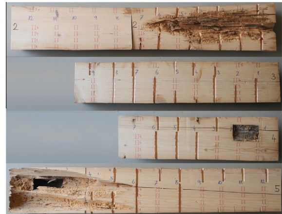
Fig. 20. Longitudinal sections four samples of tie beam [26].
