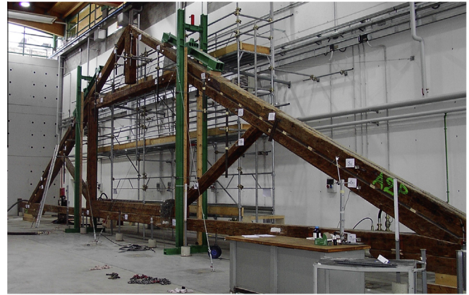
Fig. 30. The queen-post truss of “Teatro Sociale” (Trento, Italy) [35].
