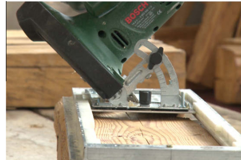
Fig. 2. Circular saw with guides, modified.
