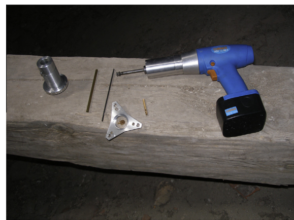
Fig. 11. Equipment for sampling of radial cores.
