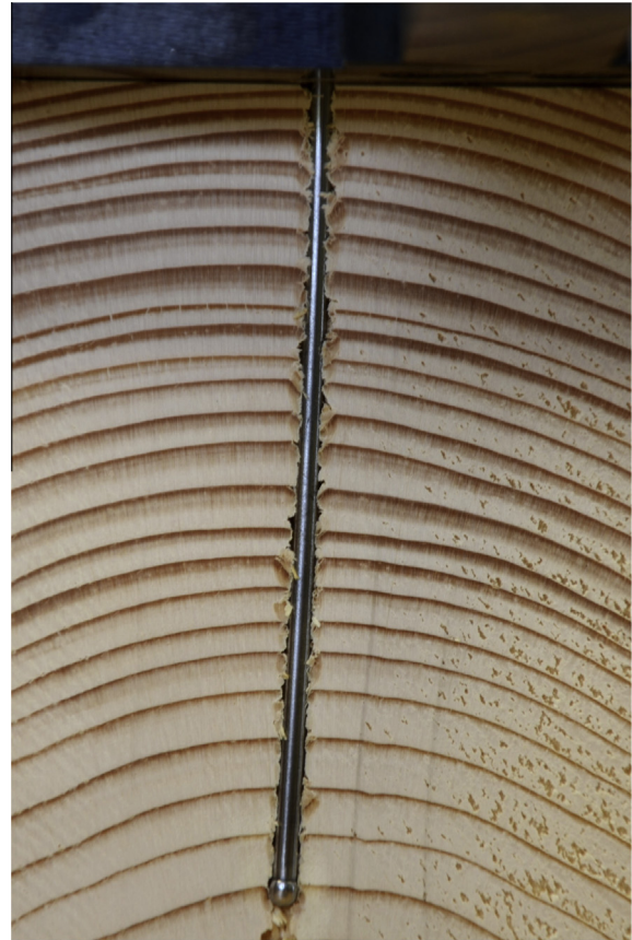
Fig. 22. A detail of pin penetration through the device base during pin pushing.
