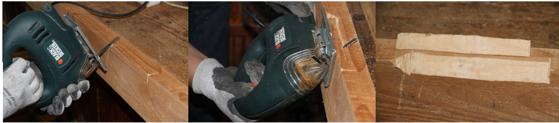
Fig. 6. Extraction of mesospecimens using a jig saw.
