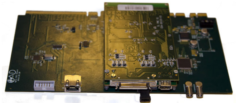
Figure 2. The Opto-Fec card with the OptoRx mezzanine plugged into it.
