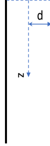
Figure 6.8: Semi-infinite tube of radius d . The z -axis originates on the tube entrance and is oriented downward [154].
