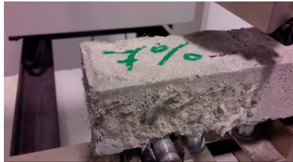
Fig.12. SW7_1 specimen. Surface not linear due to wool fibres grouped.
