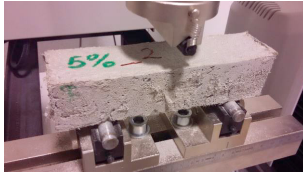
Fig. 11. SW5_2 specimen during a three point flexural test.
