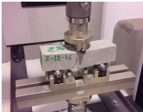
Fig. 10. Three point flexural test on SW2_2 specimen.
