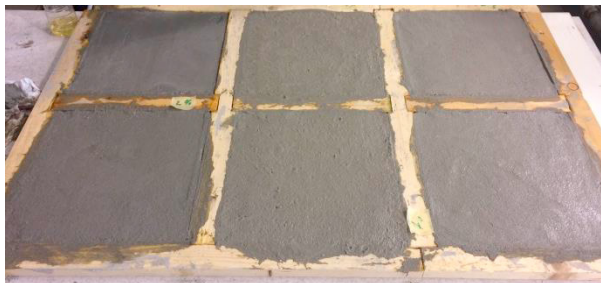
Fig.6. Thermal test specimens in wooden formworks.
